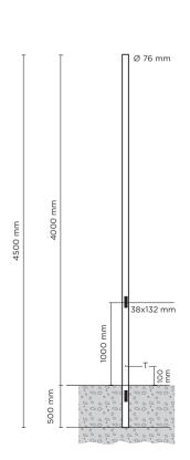
T= Grounding, threadhed galvanized insert pole Thickness= 4mm
