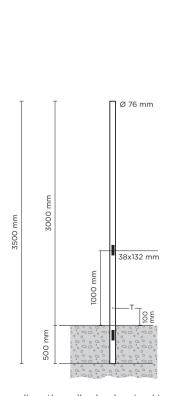
T= Grounding, threadhed galvanized insert pole Thickness= 4mm
