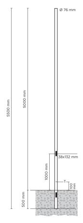
T= Grounding, threadhed galvanized insert pole Thickness= 4mm
