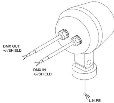
**Wiring diagram for RGBW version:**
