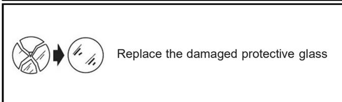
Replace the damaged protective glass
